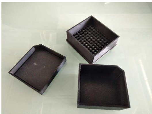
Figure 12. SEAR accessories: soil cuvette (left), press (right), sieve (back).
