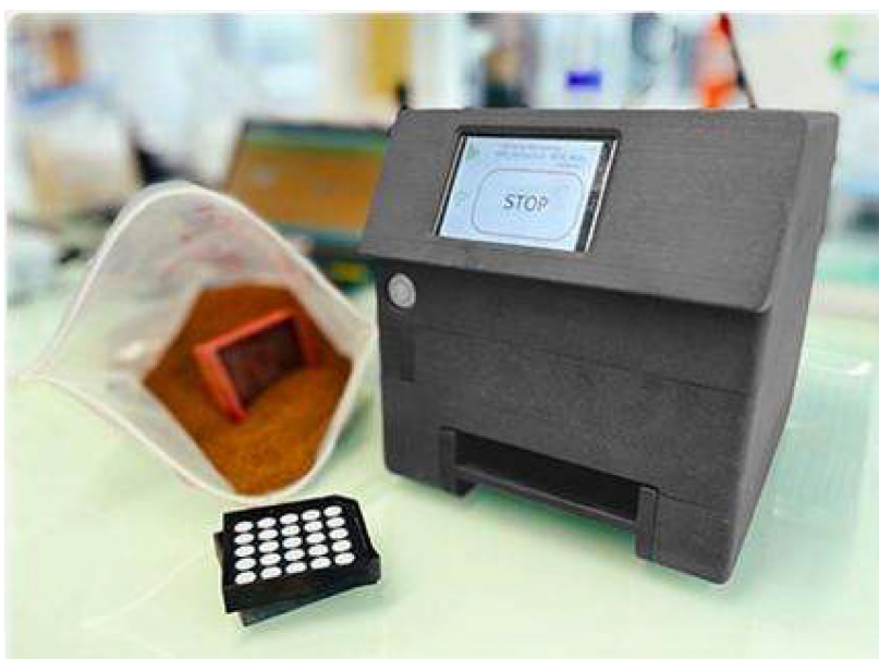
Figure 11. SEAR sensing system: reader body (right), cuvette with a reaction plate on top (middle).
