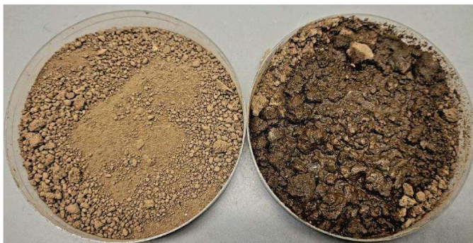
Figure 7. Dry and moist soil samples have visible differences that also affect the spectral signatures.
